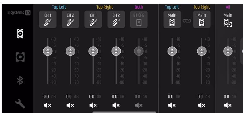
After a successful linking process, all channels of both **ICOA® PRO** devices are displayed and accessible in the **ICOA® PRO** app.
